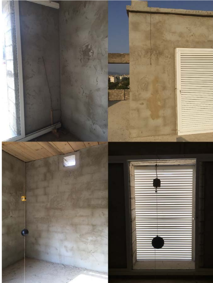
Figure 6.3 The tiny tags +2 data loggers with the inside and outside surface probes, and the ambient and radiant air temperature hanging on a thread in the middle of the room at different heights.
