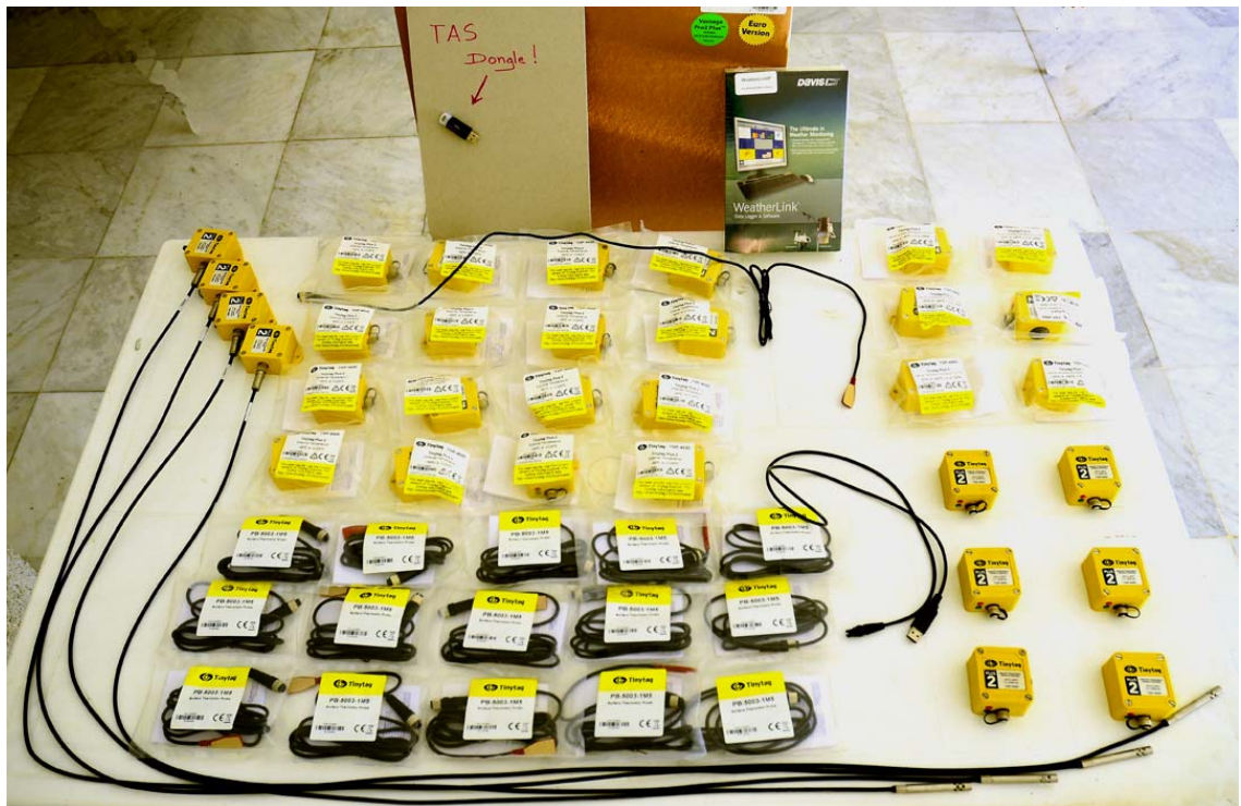
Figure 4.3 All the data loggers (old and new; Tiny Tag) and surface temperature and temperature probes.
